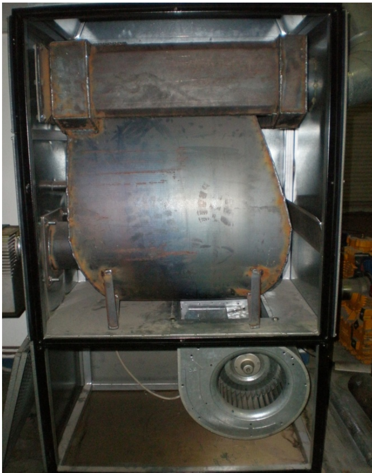
Figure 14 Exposed heat exchanger surfaces of the 30,000 kcal / h air furnace after the new position of the fan and the removal the front cover and the fan inlet grid.
