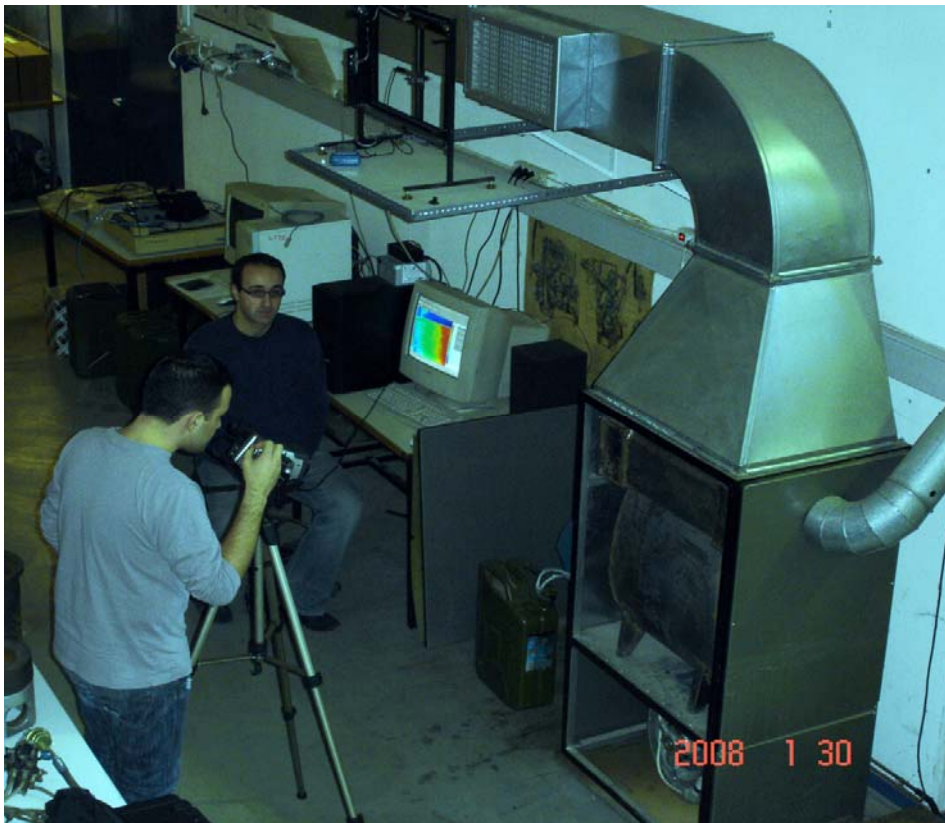
Figure 4 Measurements with infrared thermography: air furnace in operation, front panel removed. Thermocamera is shown to the left and computer with processing software at the center of the figure.
